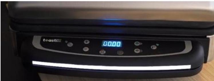
When the machine is turned on, during heating up to the maximum set temperature, the LED strip initially lights up at maximum brightness, then decreases the brightness until it switches off once the temperature has been reached.
